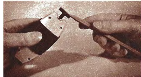
Above: Artists and draftsmen will find this pencil pointer quick and efficient. Below: The filing attachment; at 7,200 strokes per minute it does brilliant work on small objects.
