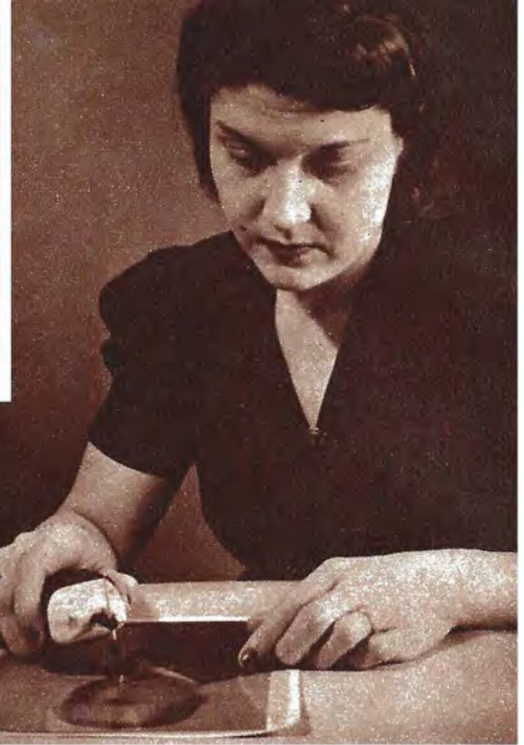
The pencil accessory will hold a needle for rapid work in dry-point etching. It may also be used for making perforated stencils.
