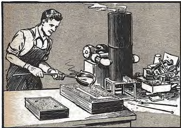
One man can easily handle this cupola. It will melt 35 lbs. of iron at a time, or about 300 lbs. per hour.
