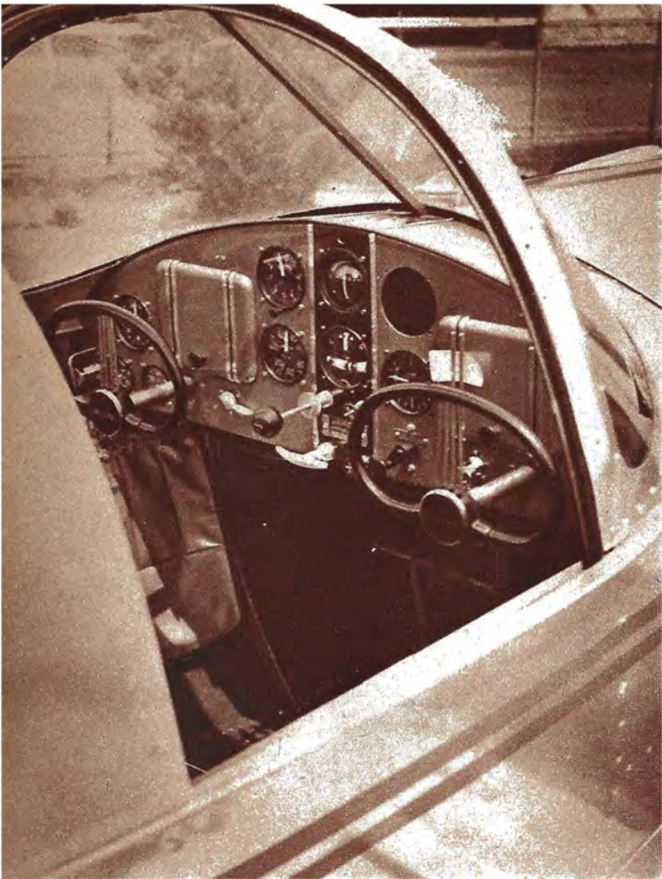
Above: The Ercoupe's instrument panel. All steering, climbing and descending is effected with the hand wheel; the feet have absolutely nothing to do. That's the throttle between the wheels. The brake is directly below it.
