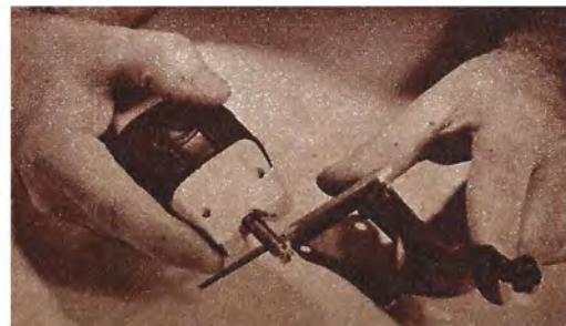
Above: Artists and draftsmen will find this pencil pointer quick and efficient. Below: The filing attachment; at 7,200 strokes per minute it does brilliant work on small objects.
