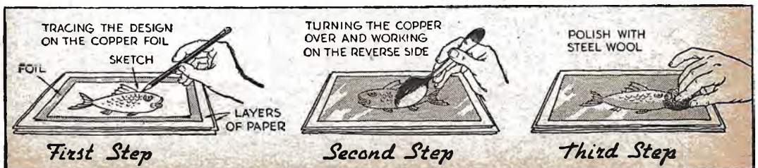
Three steps in the modeling process. Layers of paper under the foil help create a well modeled relief.
