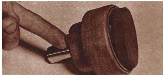
Holder for the honing stone is turned from hardwood on the lathe. Photos show parts and assembly; sectional drawing gives dimensions.
