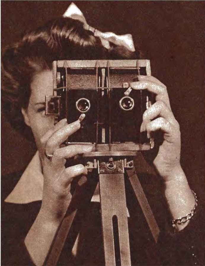
FIGURE A (above): A two-camera stereoscopic setup in use. The box containing the cameras is fastened to the top of the tripod with a small nut inset into its bottom and then glued fast. The tripod screw engages this nut. FIGURE B (below): A stereoscopic shooting setup using only one camera. The box is three inches longer than the camera. The latter makes two pictures of each scene, one from each end of the box.
