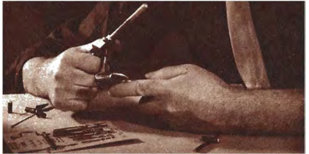
Right: A 10c tap is used to thread the accessory attachments when a set screw is required.
