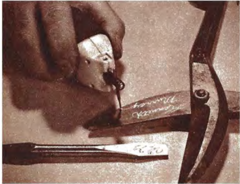
The graver attachment will write your name on tools; also use it for engraving jewelry and for cutting or ornamenting other small-sized work.
