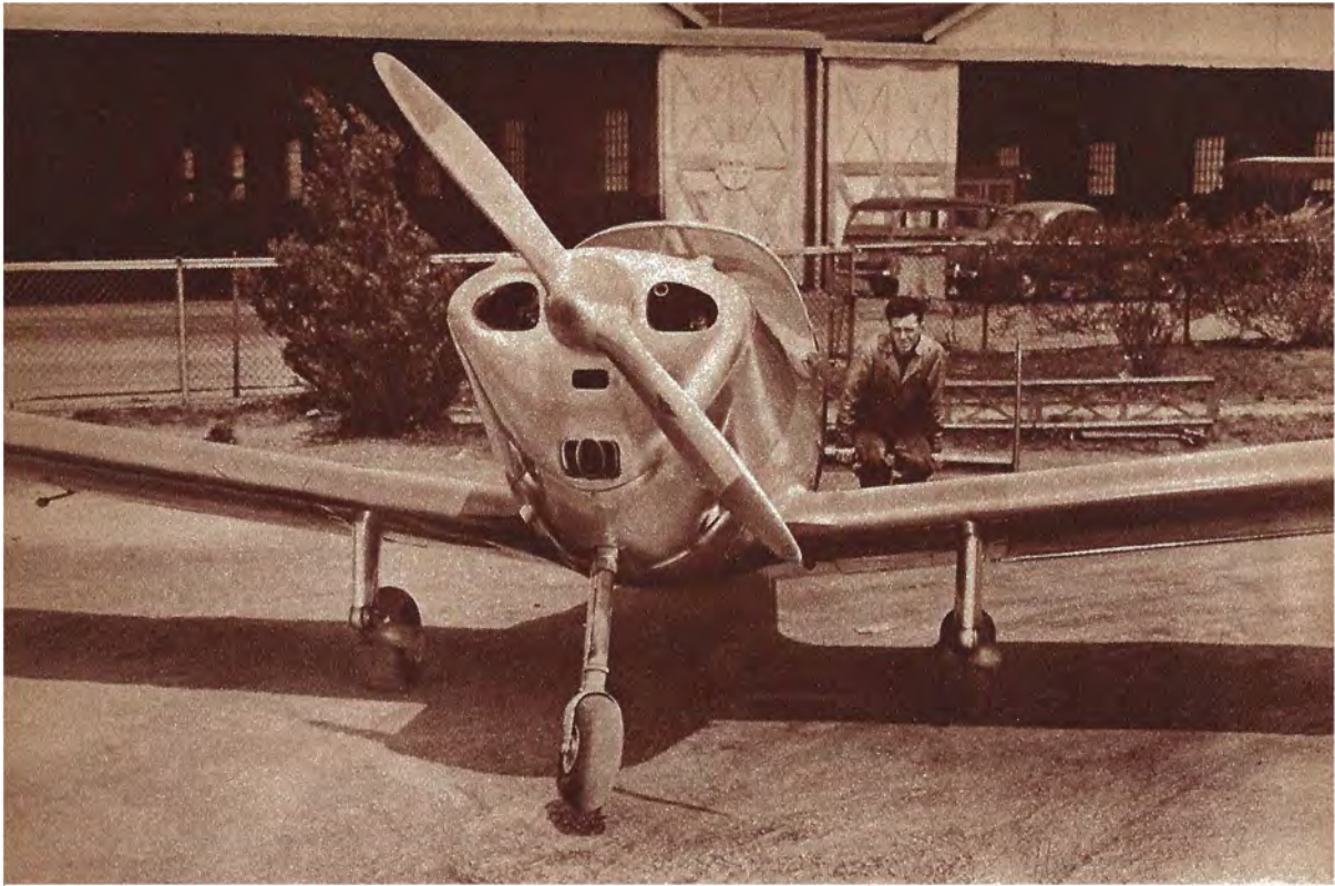
Above: Front wheel strut "stretches" like this when Ercoupe flies. Notice that it's turned to the left. Below: Engine compartment. The motor is mounted at an angle to counteract the propeller torque.
