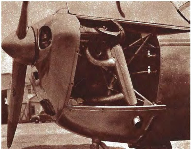
Above: Front wheel strut "stretches" like this when Ercoupe flies. Notice that it's turned to the left. Below: Engine compartment. The motor is mounted at an angle to counteract the propeller torque.
