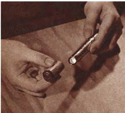
Above: Instead of fastening a piece of red tissue paper to the end of your penlight with rubber bands, for darkroom purposes, prepare the handy, removable "safety" cap illustrated. First, make a cardboard tube fitting snugly over the business end of the penlight. Then, glue or cement red tissue paper or cellophane over the free end.— L. H.
