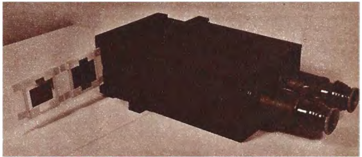
FIGURE C (right top): Component parts of the stereo viewer. It includes two telescoping boxes, and a pair of discarded field glasses. FIGURE D (right): The completed viewer with a cardboard slide holder in place in the furthestmost sliding box.
