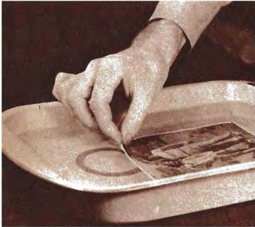
Left: Keep large, single-weight prints from sticking to the bottom of the developing tray by placing a couple of rubber jar-sealing rings on the bottom of the tray.— William Swallow.
