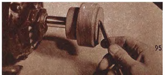
Holder for the honing stone is turned from hardwood on the lathe. Photos show parts and assembly; sectional drawing gives dimensions.
