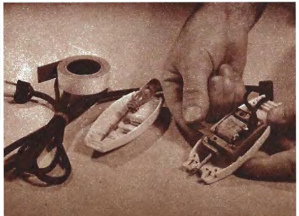
Above: Removing excess material from the plastic case, around drive shaft. Right: Thin layer of rubber tape around armature reduces stroke and quiets tool.
