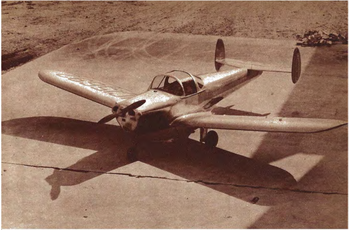
Above: This three-quarter front view shows the simplicity and low-slung lines of the little airplane. Left: On an even keel, the undercarriage looks like this. It doesn't retract. In flight, fairings streamline struts.
