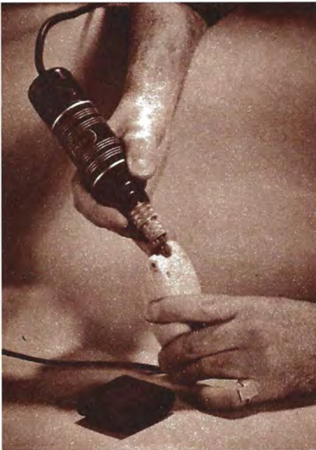
Above: Removing excess material from the plastic case, around drive shaft. Right: Thin layer of rubber tape around armature reduces stroke and quiets tool.
