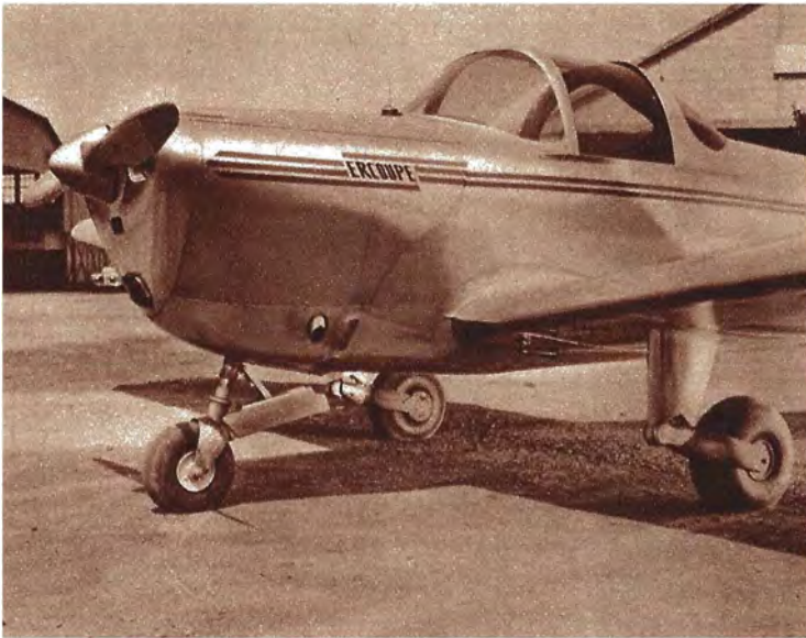
Above: This three-quarter front view shows the simplicity and low-slung lines of the little airplane. Left: On an even keel, the undercarriage looks like this. It doesn't retract. In flight, fairings streamline struts.
