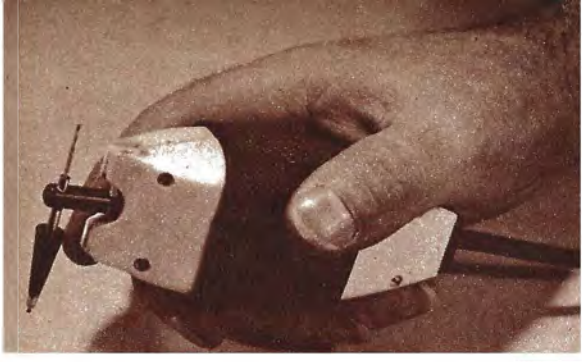
Part of a 10c automatic pencil makes up this accessory, which speeds up retouching of negatives and prints.
